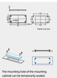
Applicable to the installation hole which has been opened, The case where the connector is not installed
